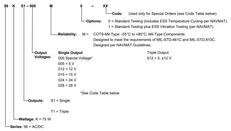
**Examples:** 56KS1-012M1 = AC/DC; 75 Watt; Single Output; +12 V; COTS-Mil-Type; ESS Vibration Testing
