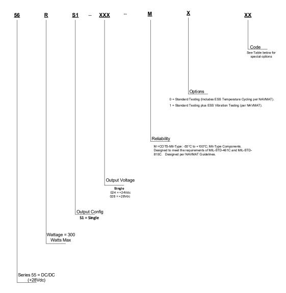
Example: 55RS1-028M0 = AC/DC; 300 Watt; Single Output; +28V; COTS-MIL-Type; Standard Testing
